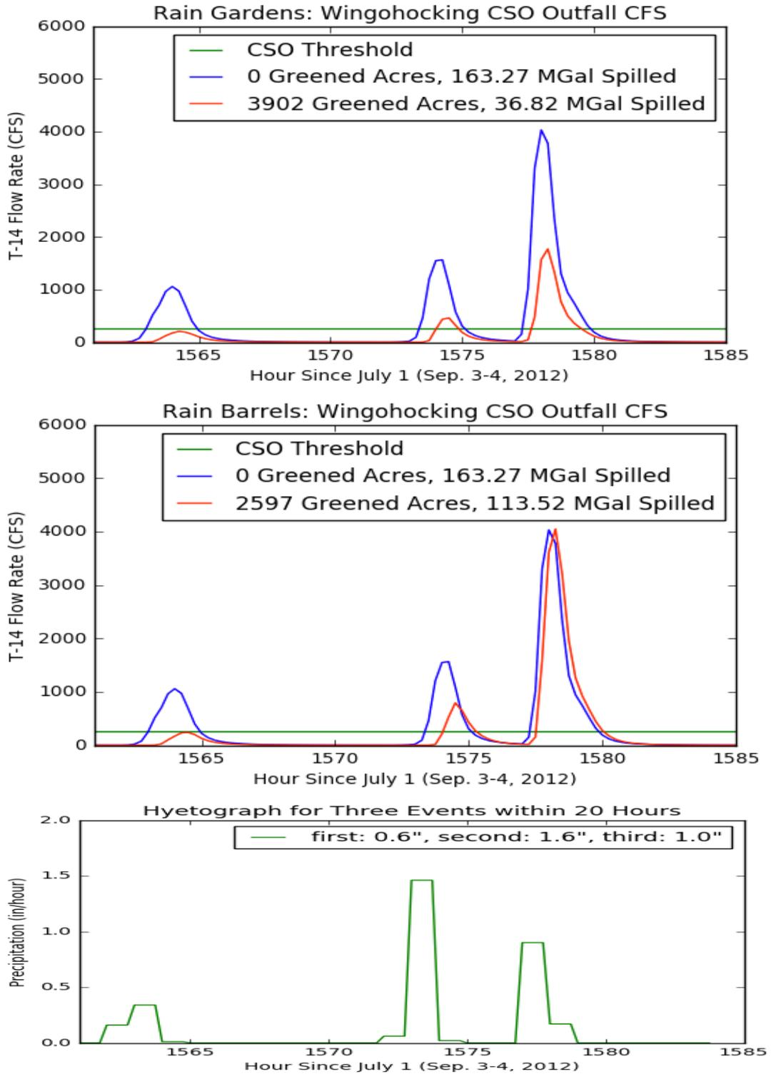
Figure 4. Time series showing hydrograph modification in the case of only rain barrels (middle graph) compared to only rain gardens (upper graph) when multiple precipitation pulses occur within 20 hours (lower graph) because rain barrels overflow when they can not fully drain.
