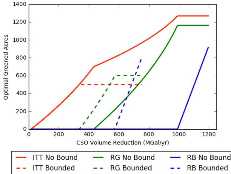
Figure 8. StormWISE results for the entire range of possible annual CSO reductions: showing greened acres to deploy of each GSI practice to *minimize total investment cost* comparing the case of no GSI bounds (Hydrological Potential) with hypothesized realistic bounds imposed on deployment of each GSI practice. Bounds assumed for these runs: ITT = 500 GA, RG = 600 GA, RB = 800 GA.
