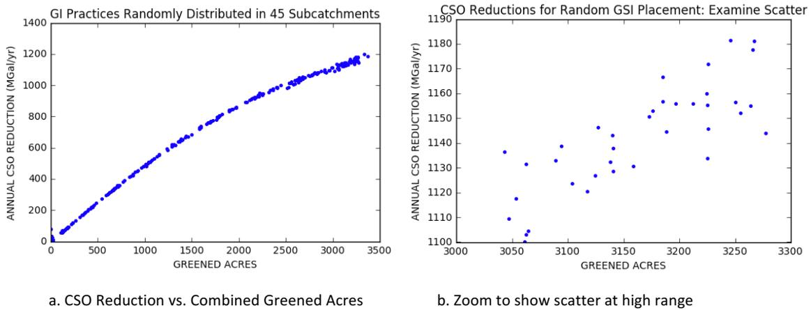
Figure 5. Results from multiple SWMM simulations with random placement of all three GSI technologies in 45 subcatchments
