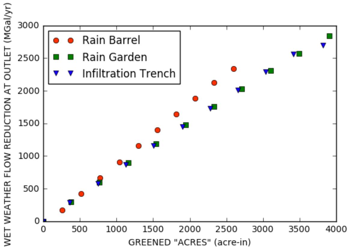
Figure 2. Results from multiple SWMM simulations: reductions in total annual wet-weather flow volumes at the sewershed outlet versus greened acres for increasing numbers of a single GSI technology deployed in the 45 larger subcatchment.
