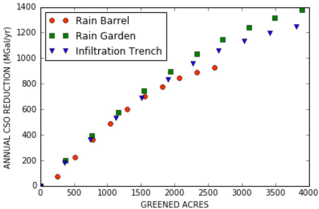
Figure 3. Further results from the multiple SWMM simulations: reductions in total CSO flow volumes at the sewershed outlet versus greened acres for increasing numbers of a single GSI technology deployed in the 45 larger subcatchments
